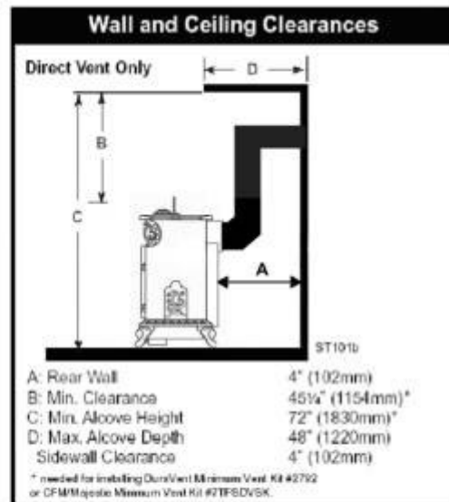
Fig. 3 Dimensions and clearances to ceiling or alcove.
