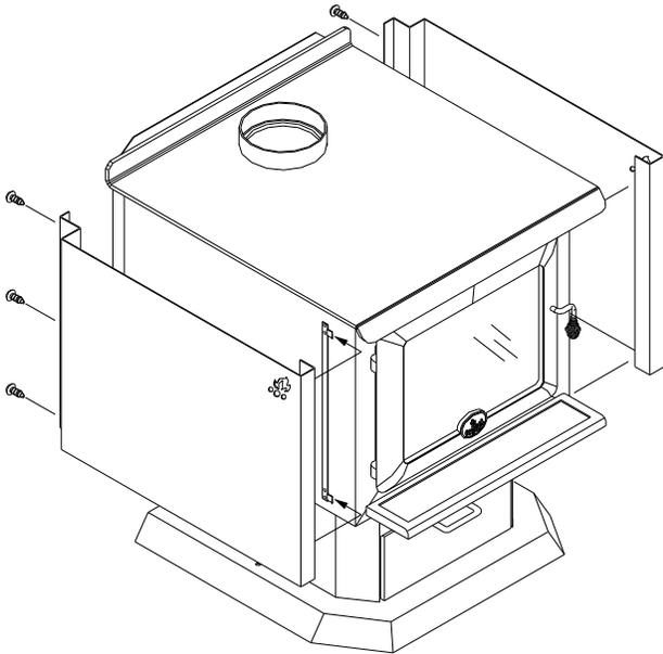
**Figure 1: Ash drawer and side shields installation**
