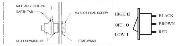
Figure 2. Earth connection installation
