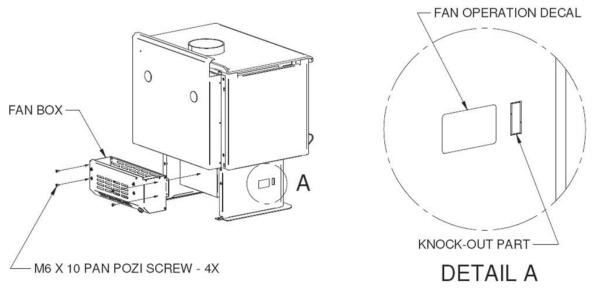
Figure 1. Pedestal version installation
