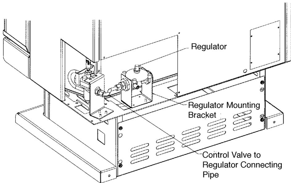
8. Connect the NG gas supply to the regulator inlet and check all new joints for gas leaks.
