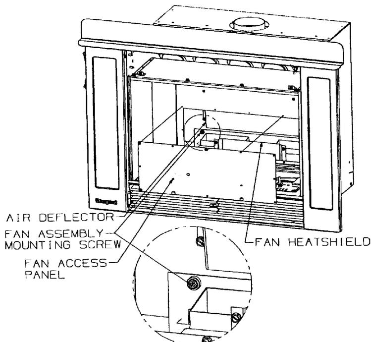
7. Release the fan by removing one screw at each end of the fan mounting plate. On later models the fan mounting screw holes are keyhole slotted, so the fan can be lifted up without slackening the screws.
