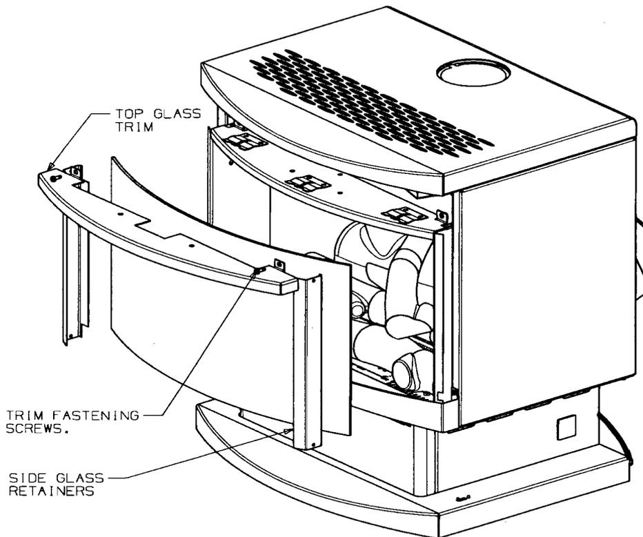
channel. Maintaining the backward pressure, slide the front glass down into the channel.
