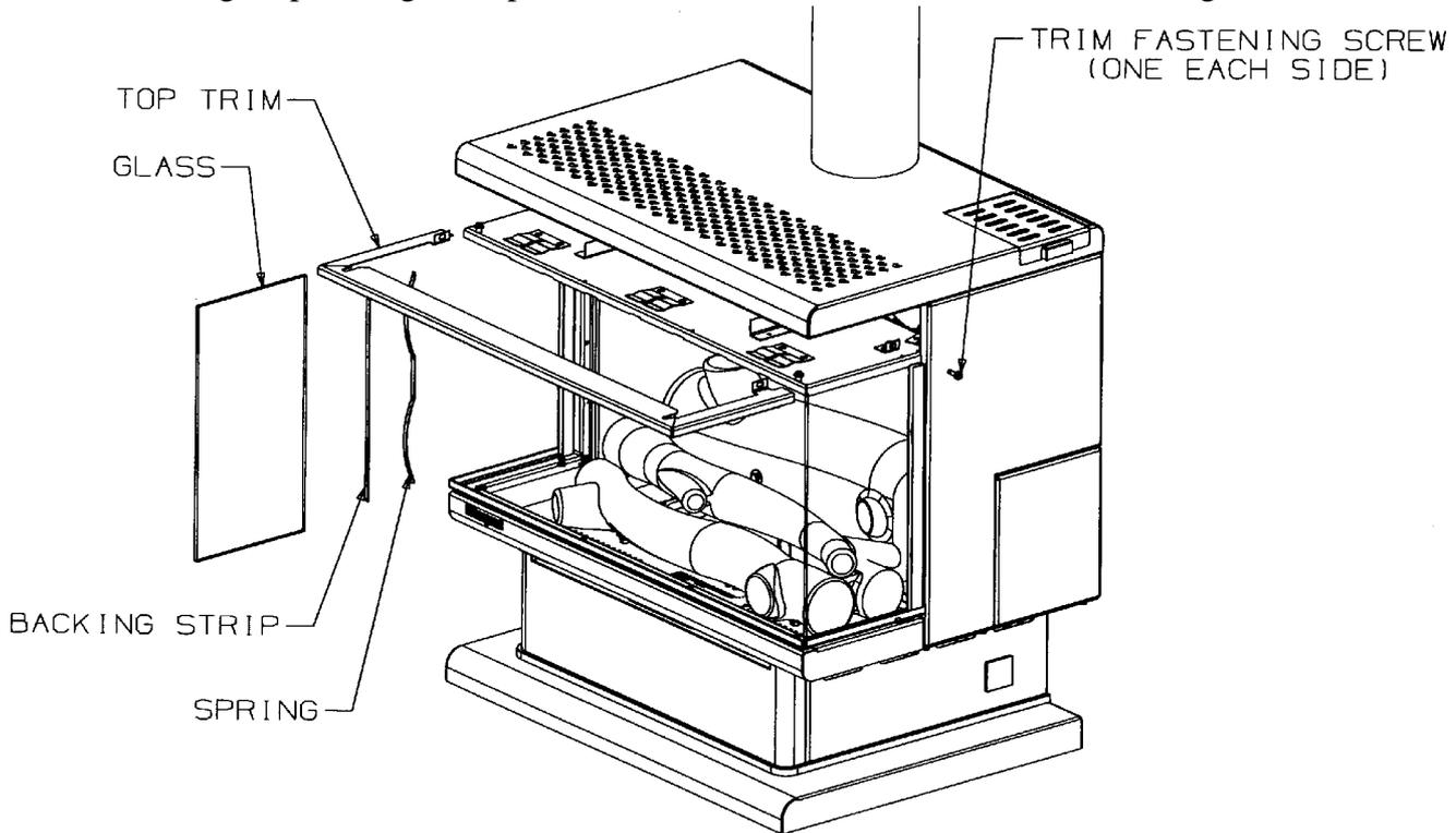
6. **Monaco.** Remove two fastening screws securing the top glass trim.
