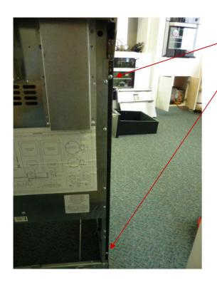
REMOVE 2X SCREWS AT REAR OF APPLIANCE
