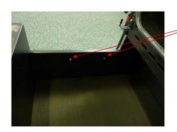
REMOVE 4X SCREWS THAT HOLD THE STORAGE DRAWER TO THE RUNNERS
