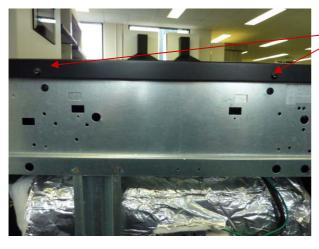
REMOVE 4 X SCREWS IN SIDE OF HOTPLATE (2 EACH SIDE )
