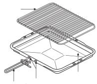
Place the handle over the edge of the grill pan, at the narrow side edges. Slide the handle to the centre, and locate between the handle position
