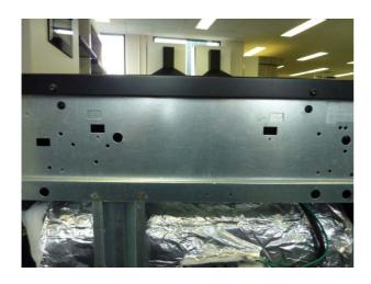
REMOVE 4 X SCREWS THAT HOLD THE ELEMNT BASE TRATY IN PLACE LIFT THE TRAY AND REMOVE THE 4 SCREWS UNDERNEATH RE-LEASING THE WARMING ELEMENT FIXING BRACKET
