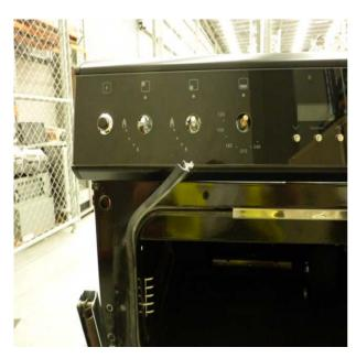
THE DOOR SEAL IS REMOVED BY JUST PULLING. IT IS SECURED IN THE GAP BETWEEN THE CAVITY AND FRONTFRAME AND REQUIRES NO OTHER FIXING
