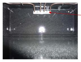
REMOVE THE 2 SCREWS SECURING THE ELEMENT BRACKET TO THE CAVITY AND PULL THE ELEMENT FORWARD TO REMOVE
