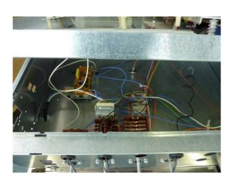
FOLLOW STEPS 4/6 AND REMOVE THE HOB TOP AND FACIA PANEL PULL THE T/STAT FROM THE SWITCH HOUSING
