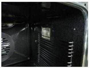
PULL OUT THE SHELF LADDERS GENTLY EASE OFF THE GLASS LAMP COVER WITH A FLAT BLADED OBJECT
