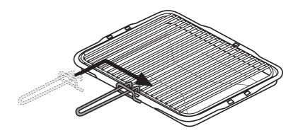
The handle should be removed from the pan during grilling, to prevent overheating. The handle is designed for removing / inserting the grill pan under the grill when grilling.
