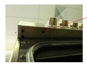
REMOVE 2X SCREWS FROM UNDERSIDE OF FACIA PANEL LOCATED AT EACH END
