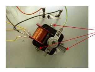
DISCONNECT WIRING FROM FAN
